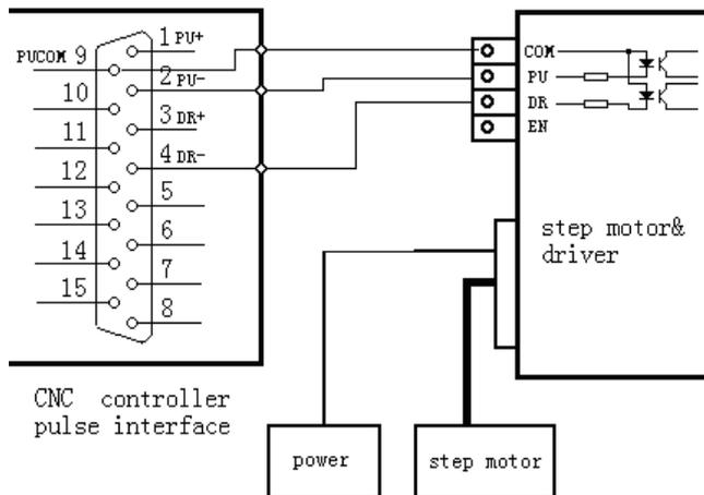
Wiring diagram to the driver of stepper motor with common anode input
