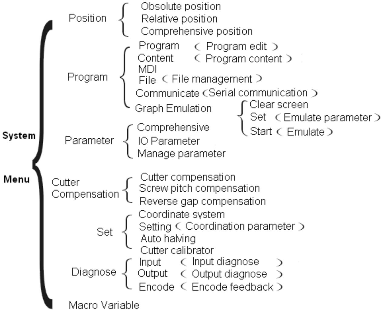
The multi-level design is adopted for the system menu. The menu operation keys, namely F1-F6, correspond to the menu options on the screen. To enter the corresponding menus, press these keys. If the menu contains submenu, the system will enter the submenu after it is pressed. If the menu is a function one, the corresponding function will be performed. The cyclic keys are used for scrolling the menu pages, whereas Menu Return is used for returning to the previous menu.
