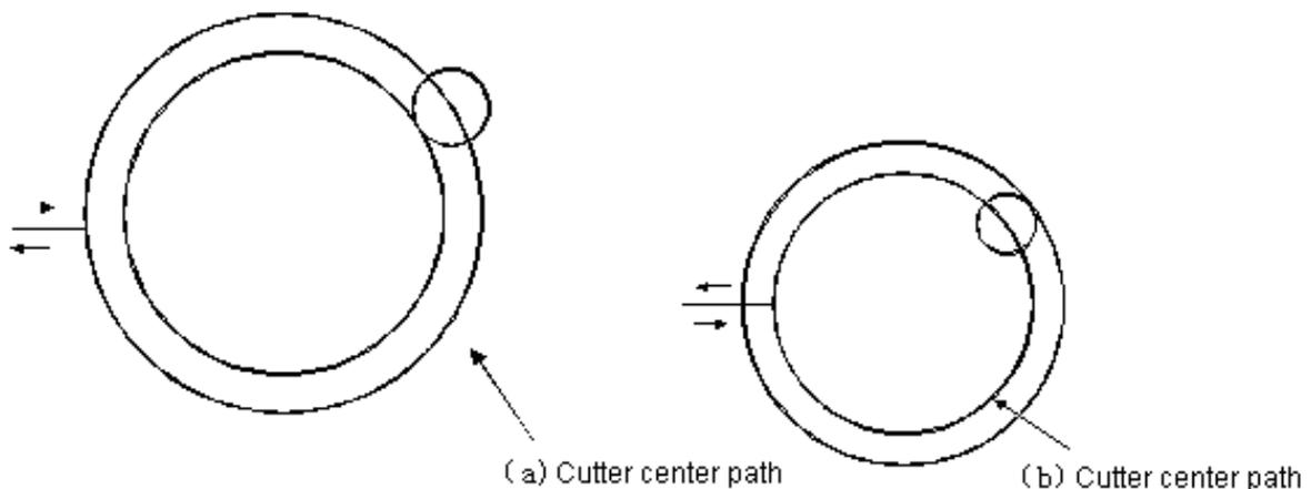
➤ **Using cutter radius to compensate excessive cutting**
