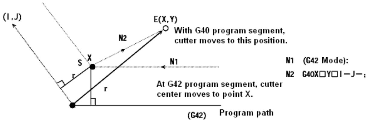
Note: The obtaining of cutter intersection by CNC is irrelevant to the inner and outer sides of the designated machining.
