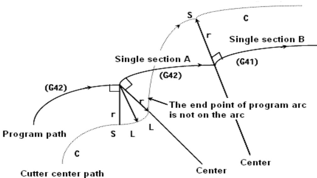
➤ When the cutter center path for cutter radius compensation is more than one circle in length
