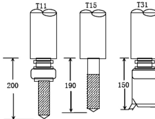
The value of offset number 11 is 200.0, of 15 is 190.0 and of 31 is 150.0. The offsets are set respectively. The program is shown as follows:
