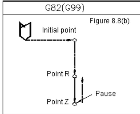
The fixed cycle of G82 has an action of pause at the hole bottom. Other procedures are the same as G81. The pause at the hole bottom can improve the precision on hole's depth.
