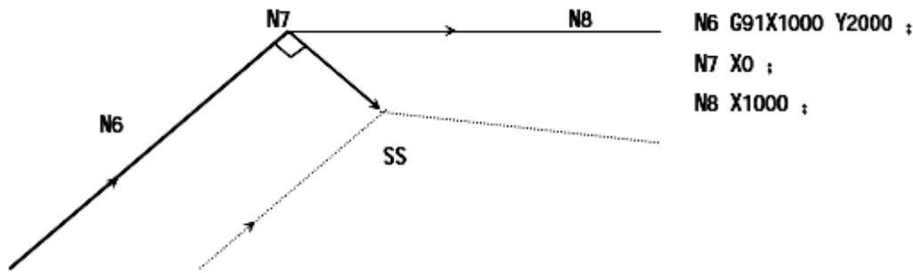
Two program segments without cutter movement can't be executed consecutively. If executed in that way, a vector, which takes the length as the compensation value and whose direction is vertical to the movement direction of the previous program segment, will be generated. This will lead to over-cutting.
