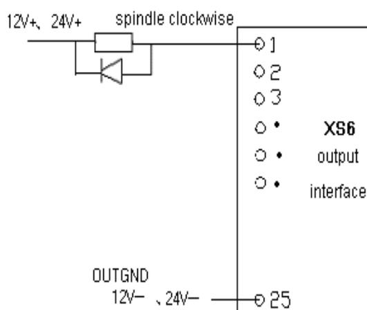
**Wiring diagram of machine(right)(take spindle on CW)**
