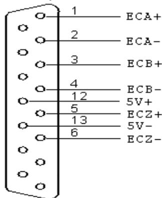
The standard wirings of Spindle encoder is suitable for CNC4240 and CNC4342 controller.
