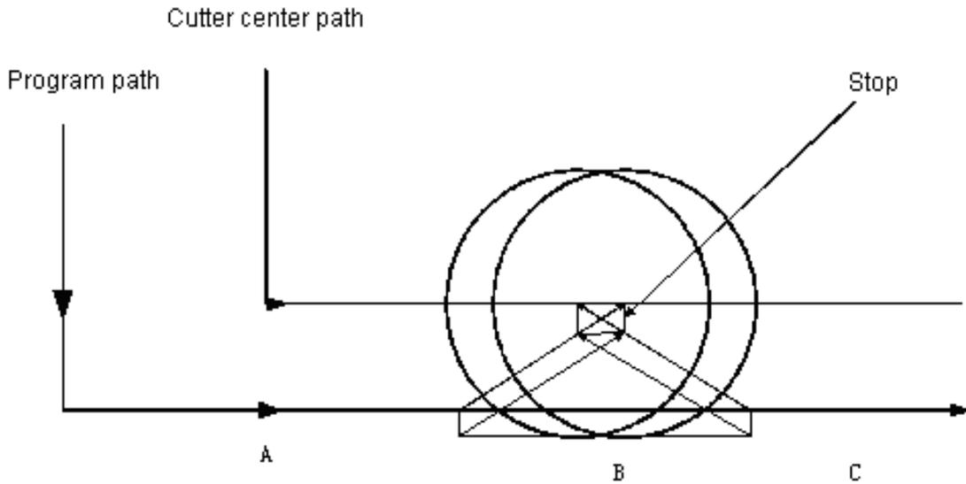
No interference actually happens. However, as it is the program segment B, the direction of program is opposite to the path of the radius compensation. The cutter will be stopped and alarm information displayed.
