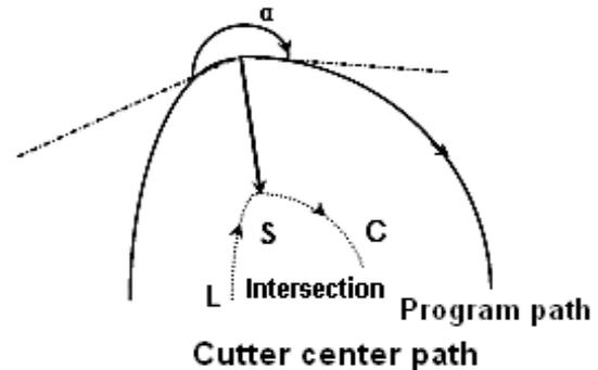
(v) Machining for inner side of less than  $1^\circ$  and compensation vector amplifying.
