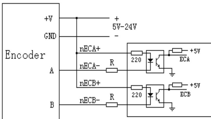
The voltage of the power supply depends on the encoder, when using 5V power supply, the resistance R is not required; when using 12V power supply, it can use 1K-2K resistance for R; when using 24V power supply, it can use 2K-5K resistance for R.
