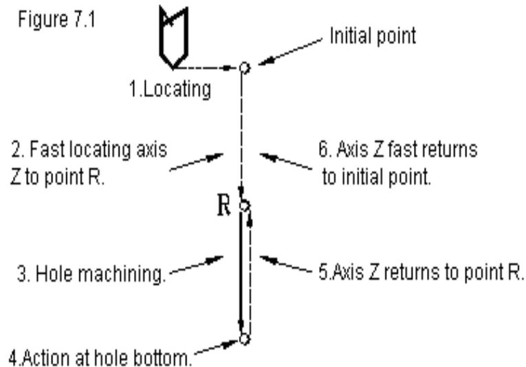
The instruction G90/G91 and G98/G99 can affect the execution of the instruction for fixed hole machining cycle. Figure 7.2(a) and Figure 7.2(b) shows the influence posed by G90/G91 to the instruction for fixed hole machining cycle.
