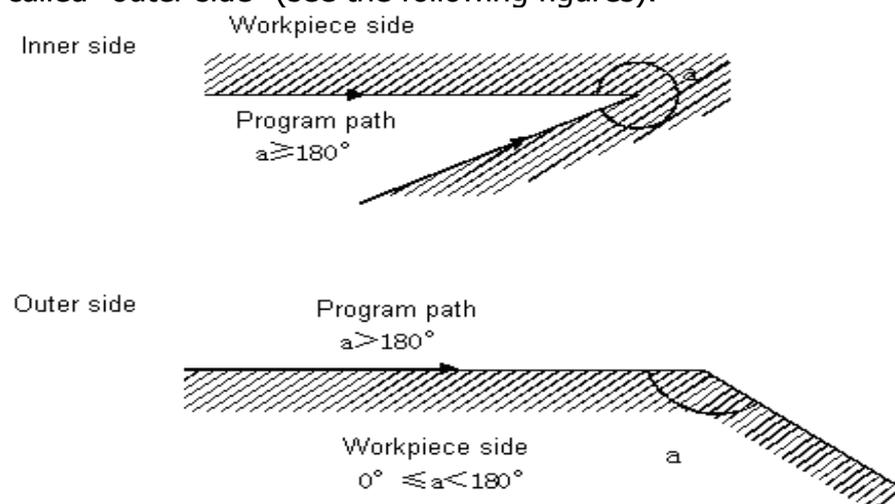
(a) Move along the inner side of the corner ( $\alpha \geq 180^\circ$ )
