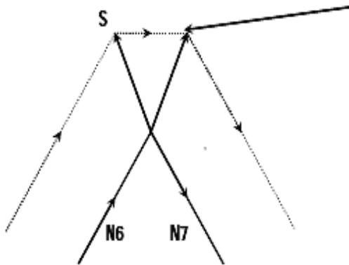
These movements belong to the program segment N7. Therefore, the feedrate equals that of the program segment N7. If program segment N7 is of G00 mode, the cutter will move at the fast feedrate. If of G01, G02 and G03 modes, it will move at the cutting feedrate.
