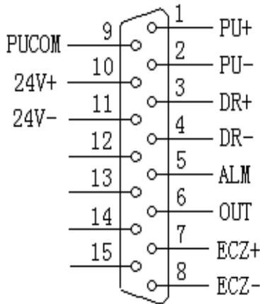
XS1..XS4pulse interface standard wiring
