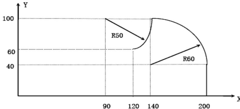
Use absolute value method and incremental value method respectively to program the locus in the diagram.
