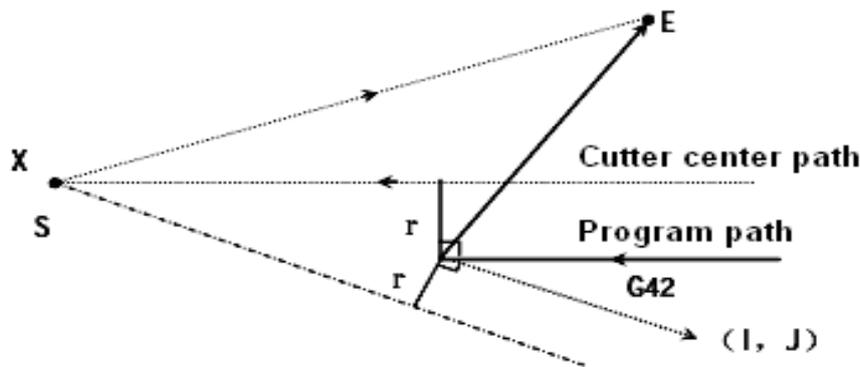
When the intersection can't be obtained, the end point cutter of the previous program segment moves to the position vertical to the previous program segment.
