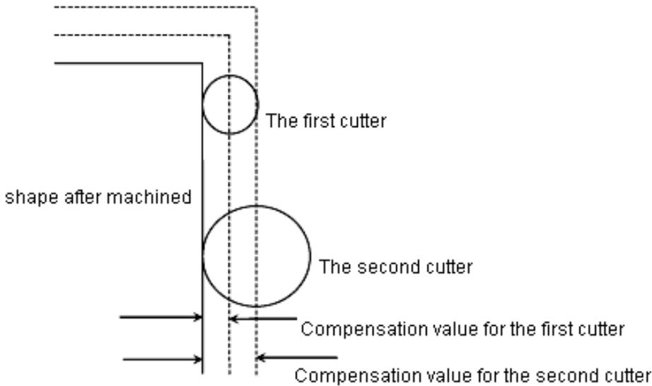
As shown in the following figure, the cutter with radius  $R$  is used to cut the workpiece  $A$ , the central path of cutter is  $B$ , the distance between path  $B$  and  $A$  is  $R$ . The process that the cutter leaves the workpiece  $A$  for some distance is called "compensation". Programmers use the radius compensation mode to produce the machining programs. In actual machining, the radius of cutter will be measured and entered into CNC. The cutter path becomes the compensation path  $B$ .
