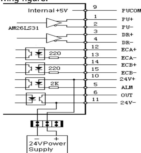
Internal Electric Diagram for Pulse Output.
