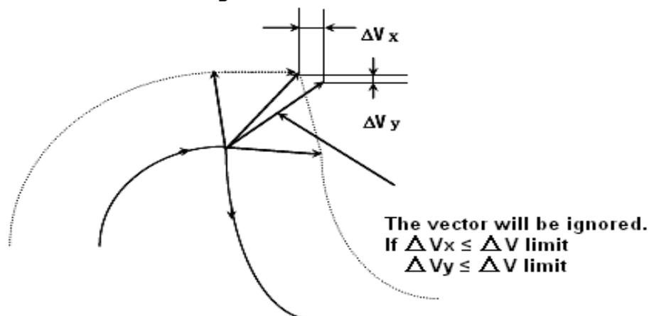
If  $\Delta V_x \leq \Delta V \text{ limit}$  and  $\Delta V_z \leq \Delta V \text{ limit}$ , the latter vector will be ignored.  $\Delta V \text{ limit}$  uses the parameter.
