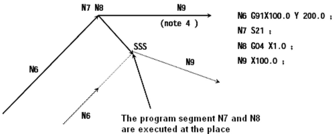
Note: SSS indicates the program segments are used for operating the cutter thrice.
