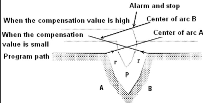
In the left figure, when cutter radius is a small value, the compensation path of arc will have intersection. However, when the radius value becomes greater, the intersection may not exist. The cutter will stop at the end point of the previous program segment and the system will display the alarm information.
