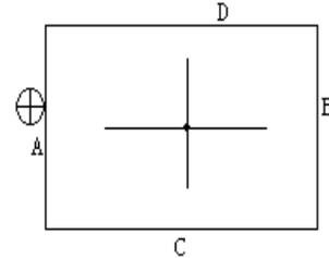
The item Halving performs the function of cutter calibrating, by which the system can automatically compute the central position of the workpiece. Through this item, operations such as line halving, rectangle halving and circle center locating can be conducted.
